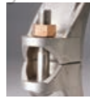
a stainless steel bolt fastened with a silicon bronze nut
